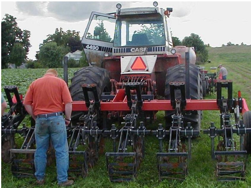
**Figure 1. Zone Builder equipment with rolling basket behind**
